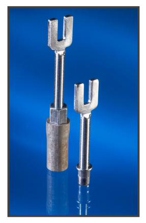
There are two plugs as shown in the image to the left. The small plug is used for depths up to 75mm and the large plug for slabs of greater depths above 75mm. A hole is drilled into the existing concrete and we suggest spacings are 1 meter apart. The small plug requires a 12mm hole and the large plug a 20mm diameter hole. The depth of the whole drilled determines the adjustment range during set up.
